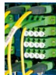
MPO connectors in order to realize ultra compact setup
